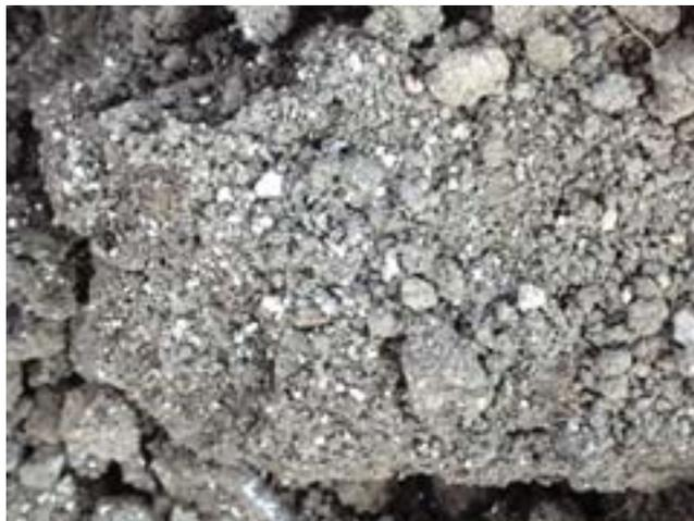
Figure 8. IXP<sup>ER</sup>® 70C Calcium Peroxide blended into treatment pile soil
